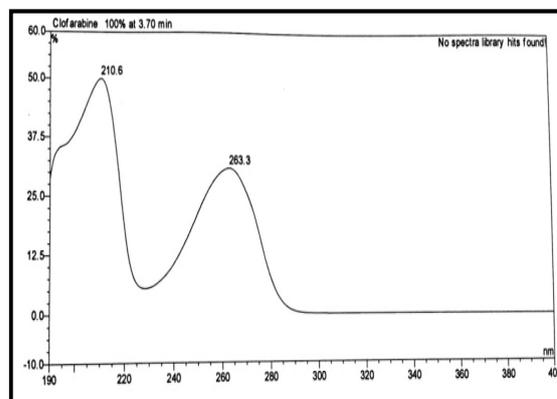
**Fig. 4** UvSpectrum of Clofarabine Assay preparation showing selection of wavelength detection
