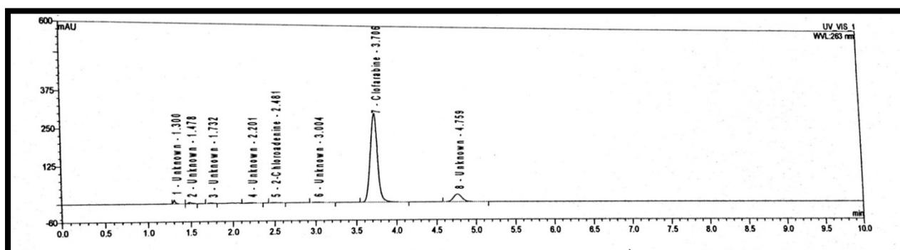
Fig. 15 Test Chromatogram of Clofarabine(15 µg/ml) for Basic Degradation
