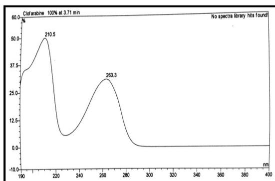
**Fig. 3** Uv Spectrum of Clofarabine Standard solution showing selection of wavelength detection
