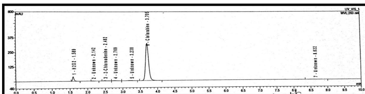
Fig. 18 Test Chromatogram of Clofarabine (15 µg/ml) for Oxidative Degradation
